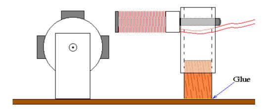
If the vibration generated by the motor moves the electromagnet, wrap the inner stand with a piece of scotch tape or thin piece of paper.
