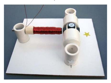
Wire comparison kit allows you to compare different gauges of electromagnet wire and experiment how different wire diameters affect the performance of the motors. These experiments can be performed with all of the motors.
