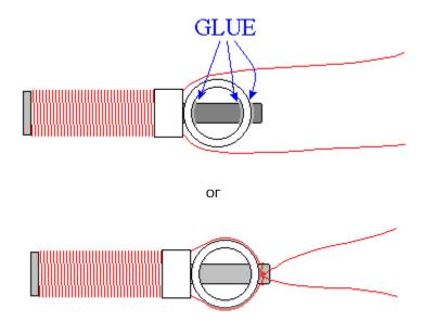
3. Place the electromagnet on the board as shown below. Turn the rotor slowly to see if the magnets hit the electromagnet. If one or more do, move the electromagnet back until there is a 1/16" (1.5 mm) gap between the electromagnet and the closest magnet on the rotor. Glue the inner stand to the board. It will allow easy replacement of the electromagnets in your experiments.
