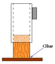
If the outer stand rotates too easy and the vibration generated by the motor moves it, wrap the inner stand with a piece of scotch tape or thin piece of paper. If you are having difficulties inserting the inner stand you may need to sand it slightly with the sandpaper.
