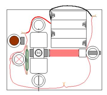
Speed control kit is a variable speed unit for the reed switch motors. It works with kits #1-5 and 8-9 and may work with any reed switch motor you built yourself. This kit allows you to control and gradually change the speed of the motor from a complete stop to the maximum speed. It will even increase the normal speed of the motor 10-25%.
