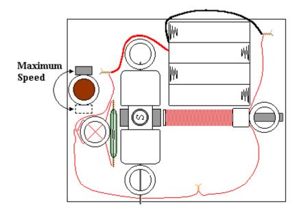
4. After you find the best position for the unit, glue the inner stand to the board as shown below. The inner stand allows the rotation of the outer speed control stand.
