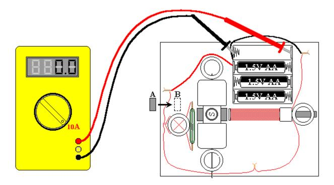
2. Glue the magnet to the speed control stand. Once again, if the magnet is oriented properly, the consumed current should decrease when the magnet approaches the reed switch.
