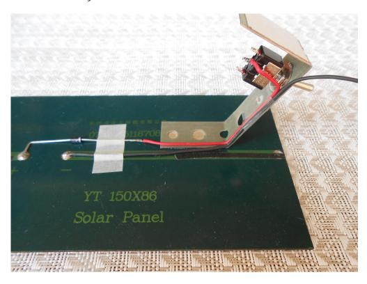
4. Attach the bracket to the board using included screw, washer and a nut. If you order the solar panel with the motor kit your board will have a countersunk hole; if you buy it separately you need to drill a hole for the screw (1/8 – 3/16" or 3.2 – 4.8 mm diameter).
