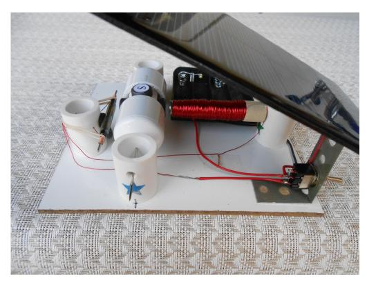
6. Connect the remaining wire from the solar panel to negative wire from the battery holder.
