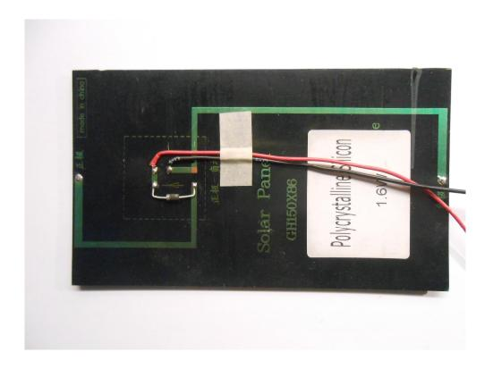
3. Attach the bracket to a solar panel. Assemble the switch on the bracket. Solder the wire from the Schottky diode to the middle point of the switch and tape wires to the bracket.
