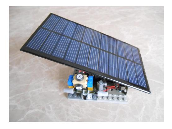
You may use 3 or 4 AA rechargeable batteries. For 3 batteries you need to use a jumper wire in the battery holder. We recommend using NiMH (Nickel-Metal Hydride) batteries; do not use Lithium-ion or any other expensive batteries.
