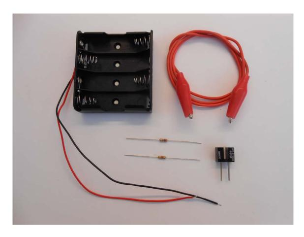
RPM Measurement Attachment comes unassembled and contains a slotted optointerrupter, two resistors, AA battery holder, and a test lead with alligator clips at the ends. You will need wire stripper (or just a knife) and some tape. Electrical tape, which is available at most hardware stores for less than a dollar, is advised but duct tape, masking tape or even scotch tape may work too.
