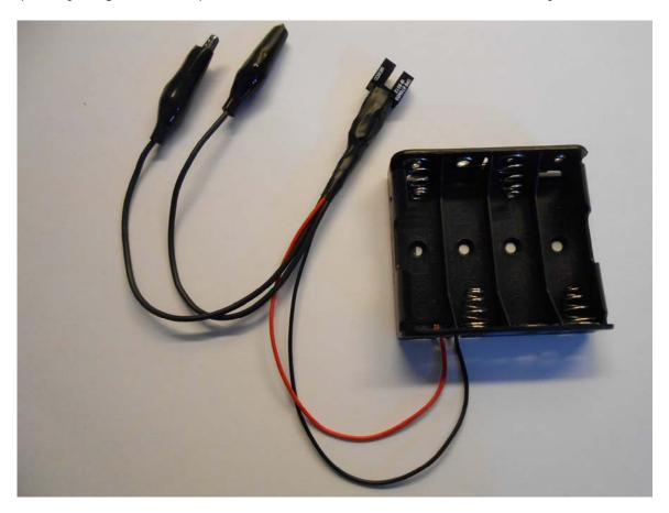
Insert four AA batteries and connect the alligator clips to the multimeter set for the frequency measurement. Yes, you need a multimeter that is capable of measuring frequency in Hertz (Hz). Not all the multimeters have this mode; if you did not order one from our site make sure that your device has it.
