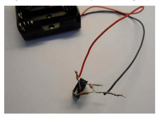
3. Cut test lead in half and strip about 3/4" (20 mm) from the ends.
