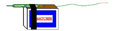
10. Put the stator (the electromagnet on the base and the books with the pins inserted) and the rotor (the cork with the needle and attached magnets) together as shown below. Position the electromagnet as close as possible to permanent magnets on the
