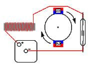
III. The magnets continue to spin due to inertia until magnet #1 gets in working range of the reed switch. It becomes magnetized again and its contacts connect together making the electromagnet push magnet #2 away.
