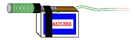
4. Using the duct tape attach the matchbox to the board as shown below.
