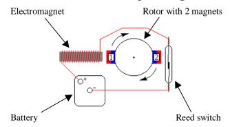
II. When the magnets spin away, the reed switch demagnetizes and gets disconnected. This creates an open circuit disabling the electromagnet.
