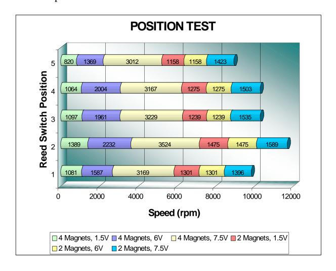
The table below shows the results of the simplified motor testing. The speed and current were measured.
