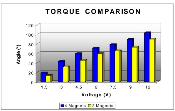
Both graphs clearly show that the rotor with four magnets outperformed the rotor with two magnets in both speed and torque experiments for all voltage settings.
