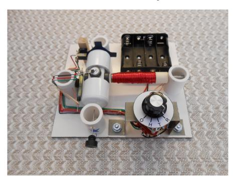
Your motors are ready to use! Keep in mind that only regular reed switch motor should work on 1.5 Volts (1 battery); all the others require at least 3 Volts.
