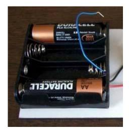
Insert the batteries and briefly connect battery holder wires to the electromagnet. If electromagnet is connected properly it should repel the magnets on the rotor turning it 45° as shown below. If it does not work – switch the wires.
