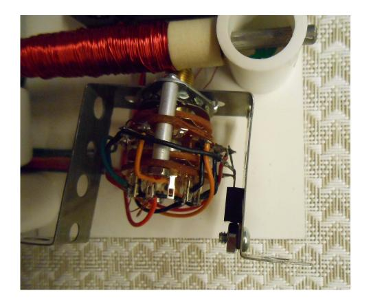
Usually the bracket provides enough heat dissipation for voltages up to 12 Volts. If you plan to experiment with higher voltages you may add a heat sink as shown:
