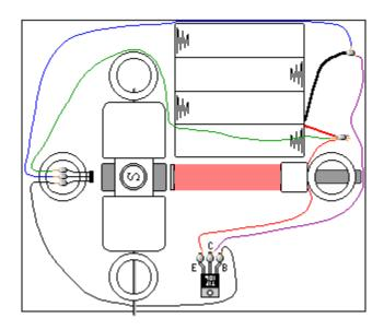
Start with 3 V. If the motor does not work, increase voltage to 4.5 V. If it still doesn't work, ensure that the rotor can rotate freely and check all the connections – it is important to clean the insulation thoroughly before soldering. Make sure the batteries are fresh and connected properly. If the motor still does not work – check Troubleshooting section of our web site.
