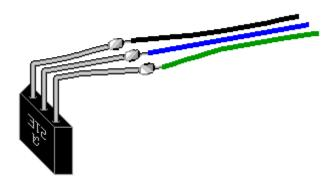
15. Insert the Hall Effect switch into its stand. Make sure that the leads of the Hall effect IC do not touch each other. You may push the wires in using a flat screwdriver.
