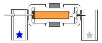
8. IMPORTANT: If you plan to attach propeller to your motor try to glue the stand with the blue star as close to the edge as possible. You may need to shift the whole rotor assembly.
