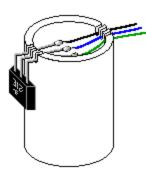
16. Glue the Hall Effect switch holder to the board. The Hall Effect switch should be located in front of the magnets at the distance of about 1/8" (3 mm) or closer. Check the rotation of the rotor to make sure that the magnets do not hit the Hall Effect switch.
