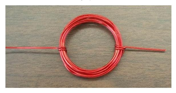
3. Strip off the insulation completely at one end and only half of it at the other. This step is very important, try to be very accurate.
