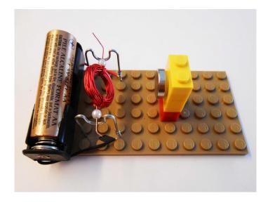
If you want to measure the speed of your motor bend the coil ends as shown. Visit <a href="http://simplemotor.com/motor-speed-measurement/">http://simplemotor.com/motor-speed-measurement/</a> for information on how to measure the speed of rotating coil in RPM.
