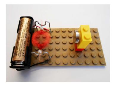
If your motor doesn't work, ensure that the rotor is balanced and can rotate freely and check the insulation. Properly removed insulation leaves shiny copper on one end. Half of the other end should also have shiny copper color while the other half should be the color of the original insulation as shown in step 3. Make sure the battery is fresh. If the motor still does not work – check Troubleshooting section at our web site at <a href="https://www.simplemotor.com">www.simplemotor.com</a>.
