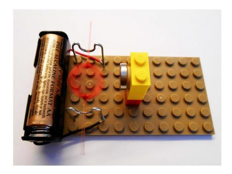
1. Leave about 3" (7-8 cm) and wind the wire 10-35 times around the AA battery. You do not have to be neat as some randomness does not affect the motor performance and may help the coil to hold its shape better. Leave 3" (7-8 cm) at the other end of the coil.
