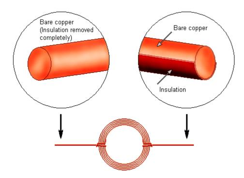
The following picture shows how to remove the insulation using the knife. Do not scratch the table - put a piece of cardboard or similar material on it. Hold the coil with one of the ends lying on the surface and remove the insulation by moving the knife in the direction shown with the arrow. Hold the blade of the knife in vertical position.
