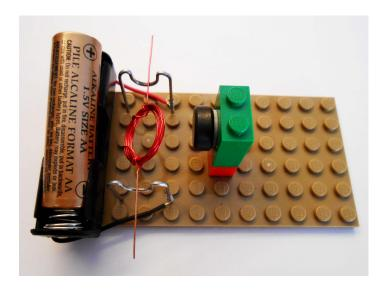
9. You may add two beads on the coil ends. These beads reduce the friction between the coil and the stands.
