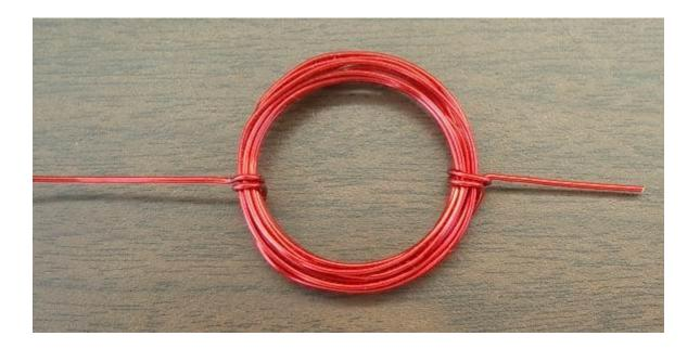
The kit contains enough wire to experiment with the coils of different size (10 and 30 windings shown).
