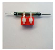
14. Assemble the reed switch on the base plate. Trim the wires as necessary and remove at least 1" (2.5 cm) of insulation.
