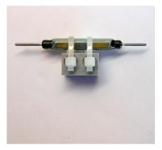
19. Assemble the reed switch on the base plate. Trim the wires as necessary and remove at least 1" (2.5 cm) of insulation.
