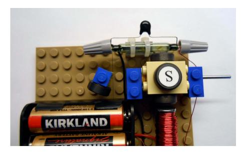
Speed control magnet counteracts with the magnets on the rotor (that is why it is important to have the same pole to face a reed switch). It changes the gap between the reed switch contacts.
