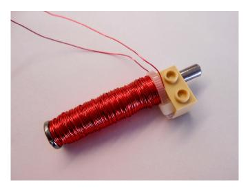
13. Remove the insulation from the wire tips with fine sandpaper (included) or a sharp knife.
