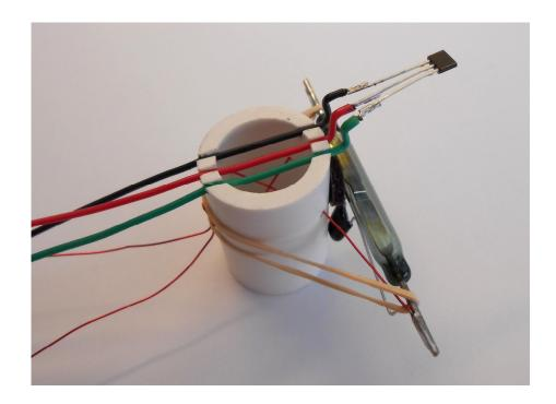
21. Glue the universal stand to the board as shown in the picture below. The Hall Effect switch and reed switch should be located at the closest distance from the magnets. Check the rotation of the rotor to make sure that the magnets do not hit any of the switches.
