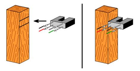
17. Attach the self-sticking felt pad to the reed switch stand as shown. This soft pad decreases the reed switch vibration thus decreasing the sound it generates.
