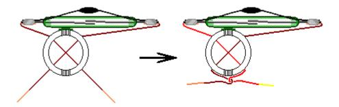
Use rubber band to prevent the reed switch from moving. The ZNR should be located below the reed switch.
