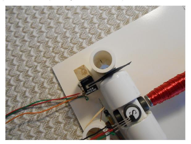
23. Attach the battery holder to the board. The battery holder allows you to experiment with 4 different voltage settings (1.5, 3, 4.5, and 6 V DC). You will need 4 AA size batteries.
