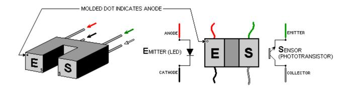
Bend and trim optointerrupter pins as shown below (view from non-branded side). Tweezers or needle-nose pliers may be very helpful. You may use scissors for trimming.
