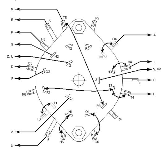
Connect connection points O3-O4, H3-H4, T3-T4, O1-O6, H1-H6, T1-T6, T5-R3 and T3-R1 using pieces of unused wires.
