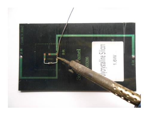
28. Solder the long piece of wire included in your kit (it should be about 13" long and is shown as black on this picture; however color does not matter) to the negative connection point on the solar panel. Solder another piece of wire to the cathode of the Schottky diode. Tape them to the board.
