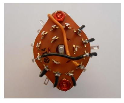
32. Temporarily attach the switch to the bracket and solder all the wires as shown below. Use the diagram from previous step with the electrical diagram from Appendix A. IT IS EXTREMELY IMPORTANT TO CHECK AND DOUBLE CHECK ALL YOUR CONNECTIONS! If you connect wrong wires the motors will not work and you may even destroy some electronic parts.
