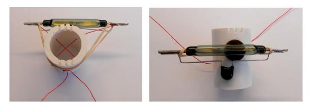
19. Bend the leads of the Hall Effect switch apart and solder three wire pieces to them. Do not overheat the Hall Effect switch.
