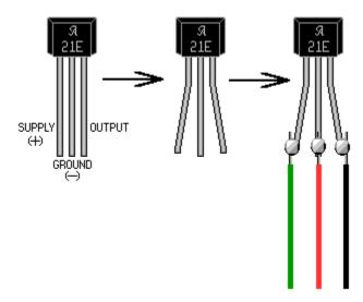
20. Insert the Hall Effect switch into the universal stand as shown below. Note that reed switch and Hall Effect switch will be controlled by different magnets to reduce the interference. Make sure that the leads of the Hall Effect IC do not touch each other and branded side is facing down.
