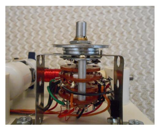
36. Attach the bracket to the board as shown on the previous picture. Before tightening the switch nut align the dial as shown below. After that align the knob with R (standard reed switch motor) and tighten the set screw.
