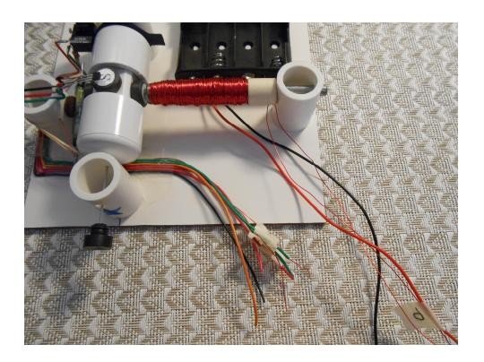
27. Assemble solar power module. Under direct sun all the motors should work without batteries; however the main purpose of the solar panel is recharging the batteries. NiMH (Nickel-Metal Hydride) batteries work great and they are being recharged even when the power switch is off.
