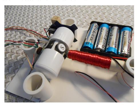
After finding the correct connection, note how the electromagnet wires are connected to the battery holder. The wire that is connected to the positive battery wire holder is marked "U" on the electrical diagram (see Appendix A) and will be connected to terminal "2" of the switch. The electromagnet wire that was connected to negative battery wire is marked "V" and will be connected to terminal "1" of the switch. Do not mix the electromagnet wires or your motor will not work!
