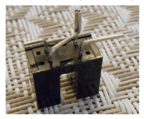
Locate the 270 Ohm and 4.7 K (4700 Ohm) resistors. The 270 Ohm resistor has red, violet, brown and gold color bands. The 4.7 K resistor has yellow, violet, red and gold color bands. Bend the leads of the resistors as shown below.
