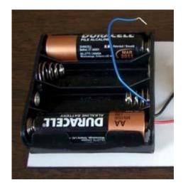
24. Insert the batteries and briefly connect battery holder wires to the electromagnet. If electromagnet is connected properly it should repel the magnets on the rotor turning it 45° as shown below. If it does not work – switch the wires.
