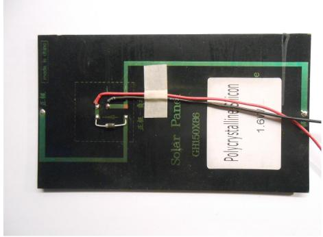
29. Attach the bracket to a solar panel. Assemble the switch on the bracket. Solder the wire from the Schottky diode to the middle point of the switch and tape wires to the bracket.
