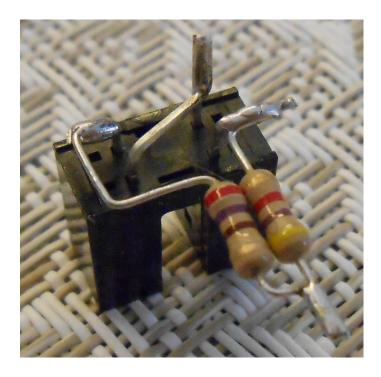
15. Solder 3 pieces of the hook-up wire to the optointerrupter assembly. If your kit includes one large piece of hook-up wire, cut it into 8 pieces of about 9" (22-23 cm) each; if it includes four 18" long pieces cut them in half. Strip about 3/8" (10 mm) of insulation on each end of these wire pieces using a sharp knife.
