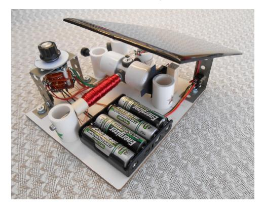
38. Attach variable speed control unit as shown. See separate instructions for the Experimentation Kit #1 for proper magnet orientation and assembly procedures. Note that speed control works only with reed switch motors.
