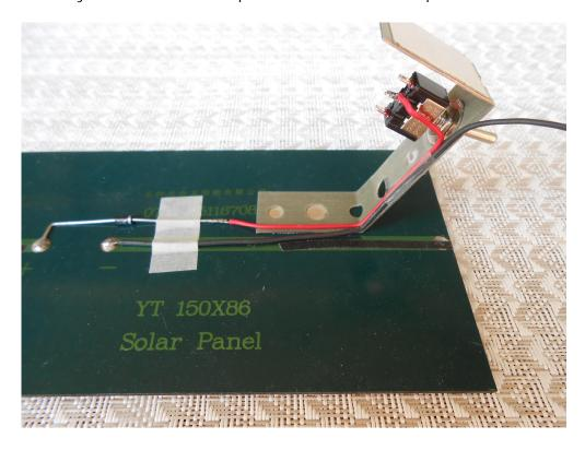
30. Solder positive wire from the battery holder to the middle point of the main switch. Solder another 9" piece of wire to the switch as shown.
