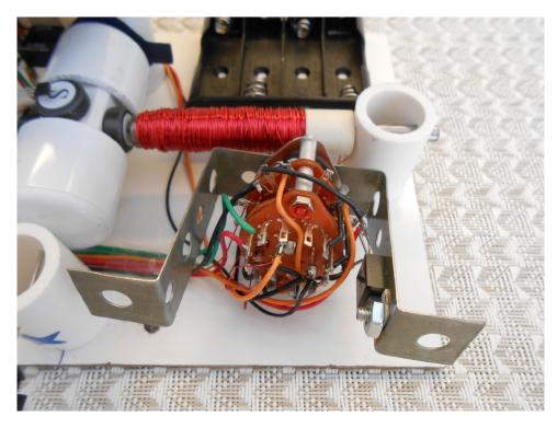
35. Tighten the knob on the switch using a set screw on the side and turn it counterclockwise until the last click, then remove the knob. Now add all the washers and a dial as shown:
