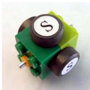
6. Assemble rotor on the base plate. Try to spin it by hand. If it does not spin freely you might need to squeeze blue bricks slightly together to push plastic shaft sleeves in. There should be a tiny gap between sleeves and inner sides of the bricks with holes.
