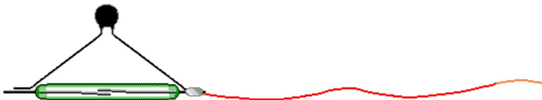
Insert the reed switch wires into the universal reed switch/Hall Effect switch stand. Be careful not to break the reed switch, it is very fragile. Twist the wires as shown below:
