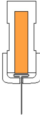
4. Insert the pushpin into the other cap until it is fully seated and the end of the pushpin sticks out approximately 1/4" (6-7 mm). You may need to push it hard.
