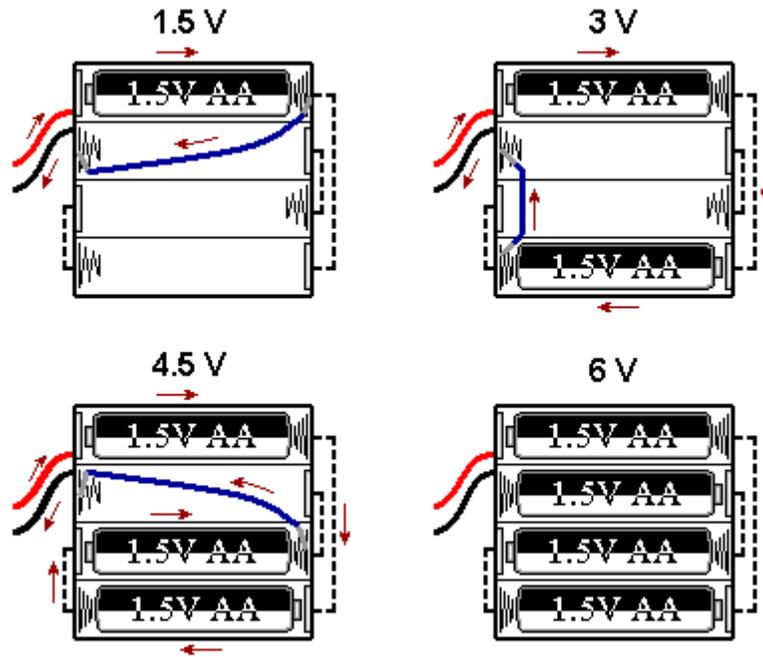
Inspect your battery holder – it may have different connections inside. In this case you can still use the jumper wire in the same manner to get all 4 voltages, but you will need to find appropriate connection points for each voltage setting.
