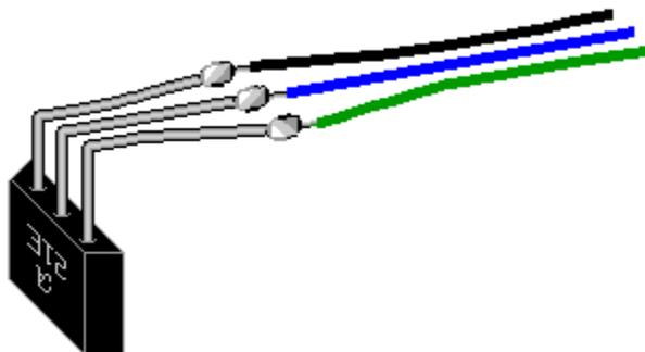
23. Insert the Hall Effect switch into the universal stand. For simplicity it is shown without the reed switch, which will be located below the Hall Effect switch. Make sure that the leads of the Hall Effect IC do not touch each other. You may push the wires into the slots using a flat screwdriver.
