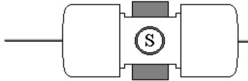
7. Cut out the disk (supplied with the kit). Poke a hole in the center, which is marked by a cross. Apply some glue to the middle of the disk and glue it to the cap with a shorter axle (with the pushpin). Slide two sequins as shown below. The sequins act as a spacer between the disk and the stand and work better if their convex surfaces face outwards. You may use only one sequin with convex surface facing the stand.
