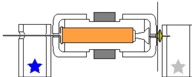
9. **IMPORTANT:** *If you plan to attach propeller to your motor try to glue the stand with the blue star as close to the edge as possible. You may need to shift the whole rotor assembly.*
