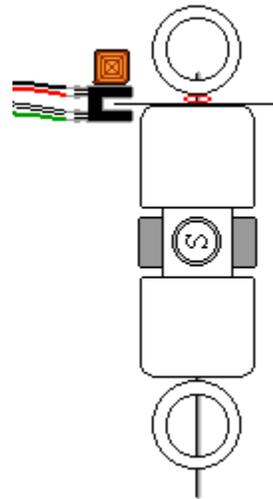
18. Attach the self-sticking felt pad to the reed switch stand as shown. This soft pad decreases the reed switch vibration thus decreasing the sound it generates.
