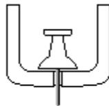
5. Put everything together as shown below. Push the caps towards each other until they cannot move any more. The T-pin must be secured firmly. This process may require some strength. Be careful not to bend the T-pin or poke yourself.
