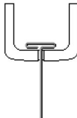
2. Insert the rotor core into the same cap as shown below. Apply some pressure to push the rotor core approximately 1/2" (10-12 mm) into the cap.
