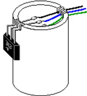
24. Glue the universal stand to the board. The Hall Effect switch and reed switch should be located in front of the magnets at the closest distance. Check the rotation of the rotor to make sure that the magnets do not hit any of the switches.
