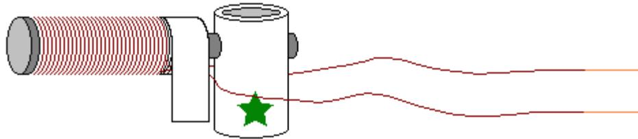
Test the electromagnet! Connect one wire to "+" and another wire to "-" of the battery. If electromagnet is assembled correctly the head of the nail should attract metal objects such as paper clips, small nails, knife blade, etc.
