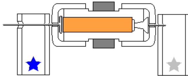
8. **IMPORTANT:** *If you plan to attach propeller to your motor try to glue the stand with the blue star as close to the edge as possible. You may need to shift the whole rotor assembly.*
