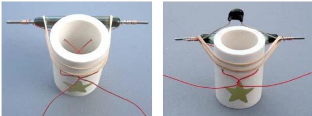
17. Glue the reed switch holder to the base. It should be located at a distance of about 1/8" (3 mm) from the closest magnet covering the gold star on the board. However, disregard the gold star position for Kit #8, as in this case the universal stand should be located in front of the magnets. Check the rotation of the rotor to see that it does not hit the reed switch.
